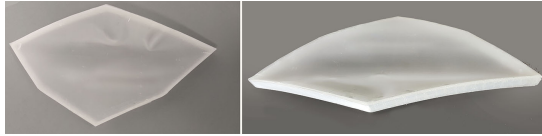
Figure 7: When cell-panels are too large, the projection paper is not able to smoothly adapt to the cell's curvature.
