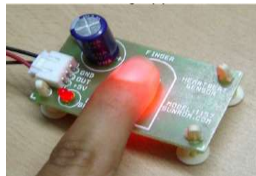
Fig 5. Using heart beat sensor
