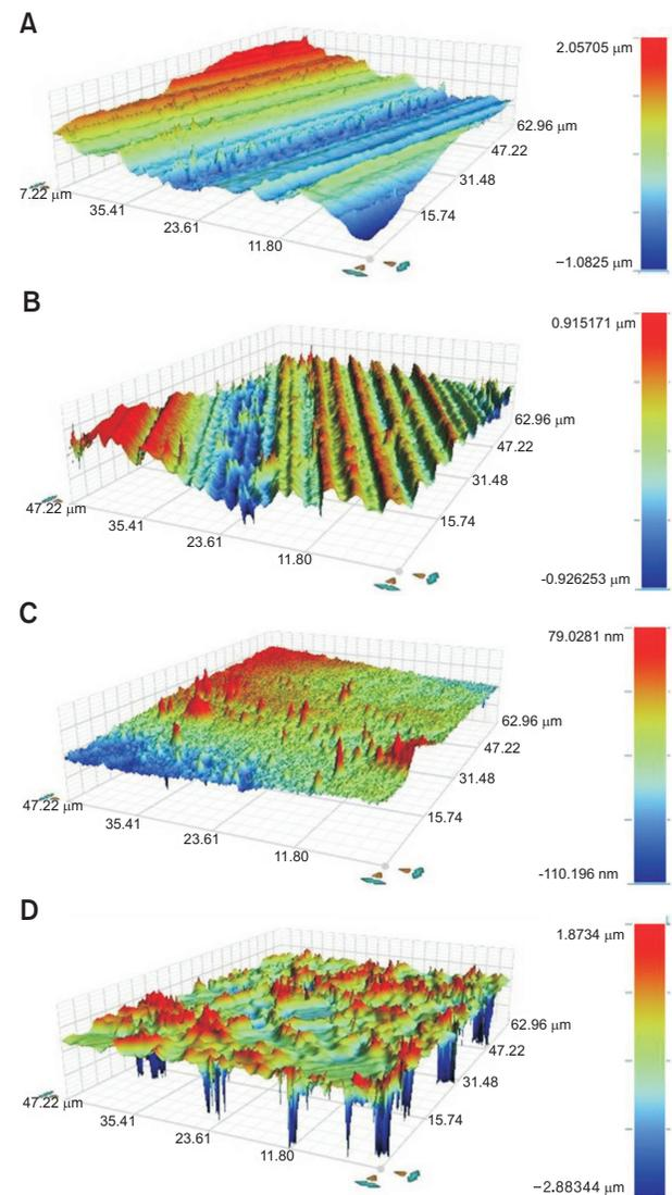
**Figure 4.** Three-dimensional optical profiler images of zirconia surface (magnification  $\times 100$ ). A, Nonglazed zirconia; B, nonglazed zirconia + sandblasting; C, glazed zirconia; and D, glazed zirconia + sandblasting and acid etching. The right side of each figure includes a colorimeter band representing the height of each spot as different color.
