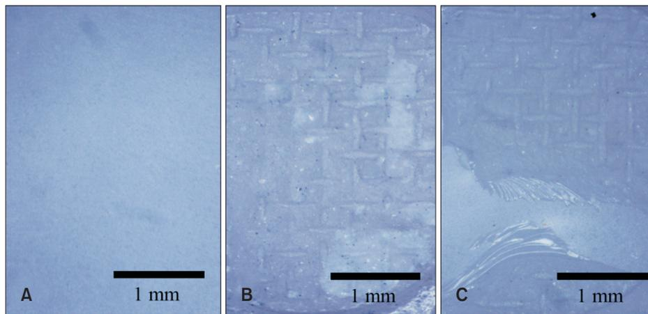
**Figure 5.** Stereoscopic micrographs of debonded surfaces (magnification  $\times 16$ ). A, Adhesive failure between zirconia and resin cement; B, adhesive failure between resin cement and bracket base; C, complex adhesive and cohesive failure.
