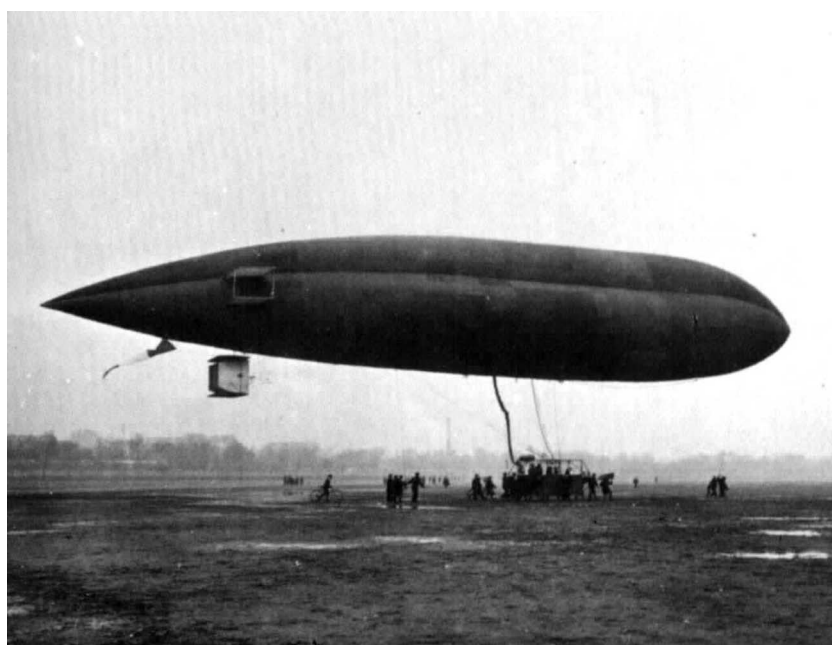
Fig. 4. Semirigid dirigible aerostat invented by Torres-Quevedo [11].
