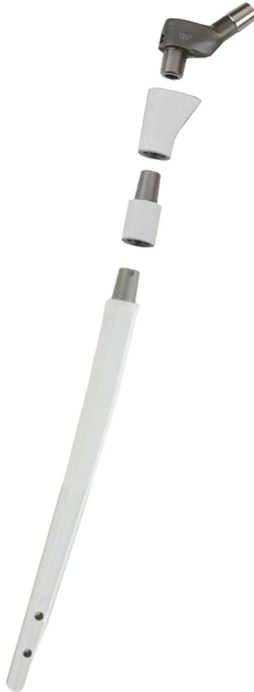
Fig 1. The modular tumor and revision system RS stem. This modular, hexagonal revision system has a hydroxyapatite (HA) coating on the metaphyseal and diaphyseal parts which allows a combined distal and proximal cementless fixation. Additionally, a non HA-coated version for a cemented fixation is available.
