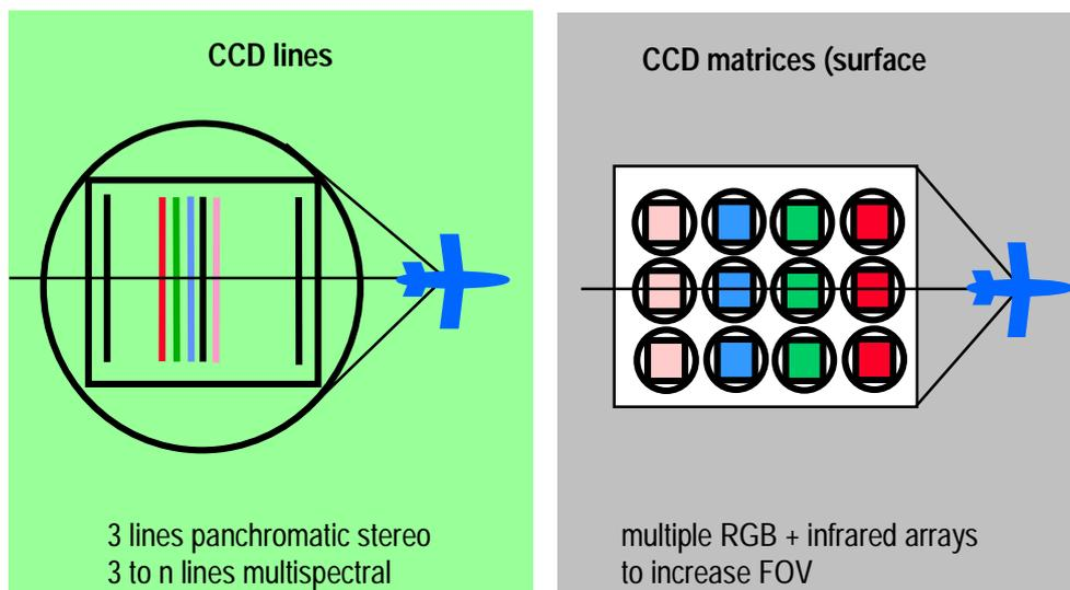
Figure 1. The alternatives: linear and area CCD arrays
