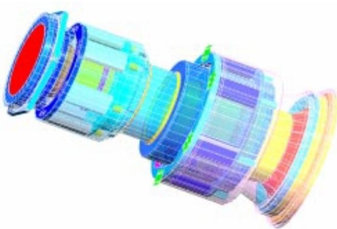
Figure 3. View of the lens of the ADS40
