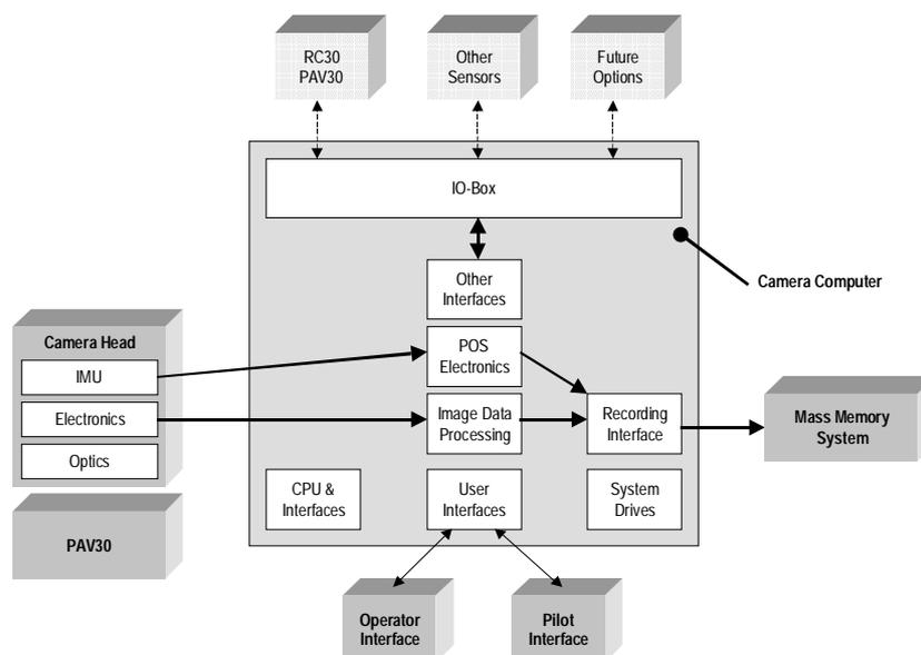
Figure 5. Components and connections of the camera computer
