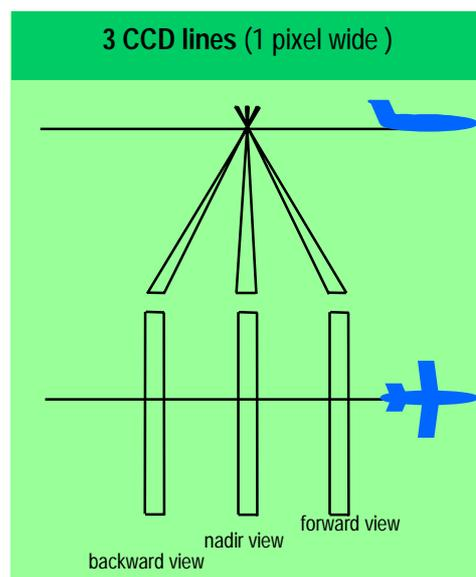
Figure 2. Basic geometric characteristics of three-line digital sensor
