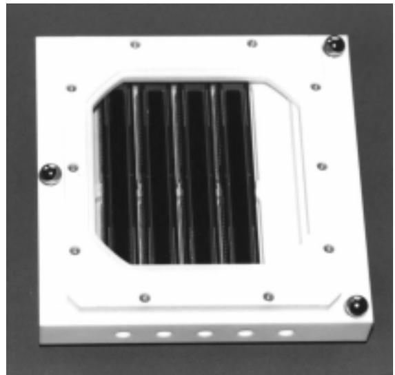
Figure 4. The focal plane module of the ADS40
