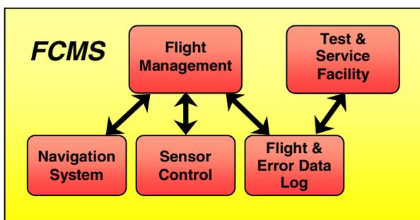
Figure 6. Components of the FCMS
