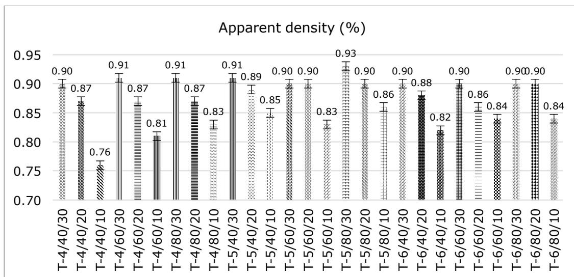
**Figure 2.** Bulk density of PP-White *Bolaina* composite materials.
