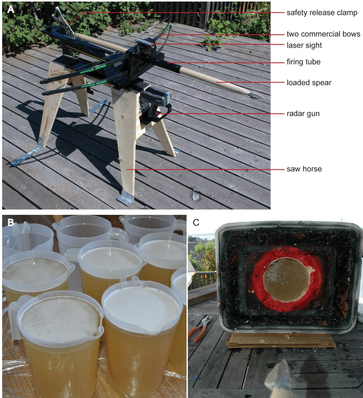
**Figure 2. The calibrated crossbow and gelatin targets.** A. The calibrated crossbow consists of two commercial bows mounted crosswise. A digital scale was used to draw the bow with a consistent 20 kg draw force. B. Fifty gelatin targets were manufactured using published ballistic standards. Plastic pictures were used as the molds. C. During shooting, the molds were secured in place with a foam target. doi:10.1371/journal.pone.0104514.g002
