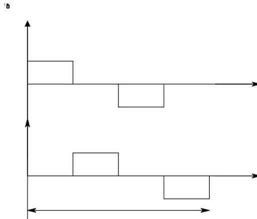
**Figure 1(a) Full step sequence of current in motor**
