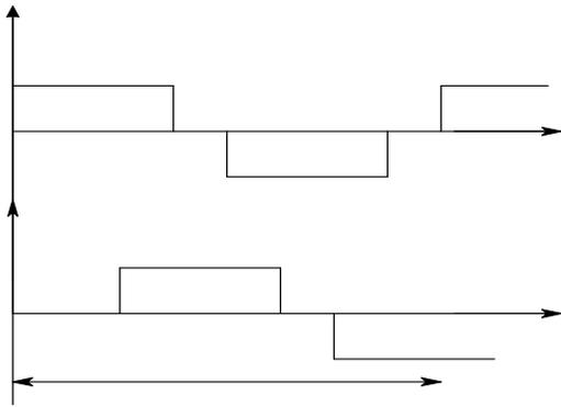
Figure 1(b) Half step sequence of current in motor
