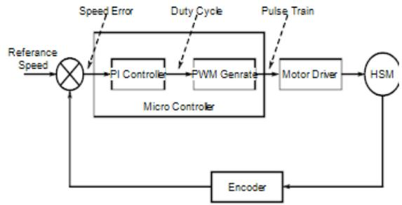
Fig.3 Speed control with encoder feedback
