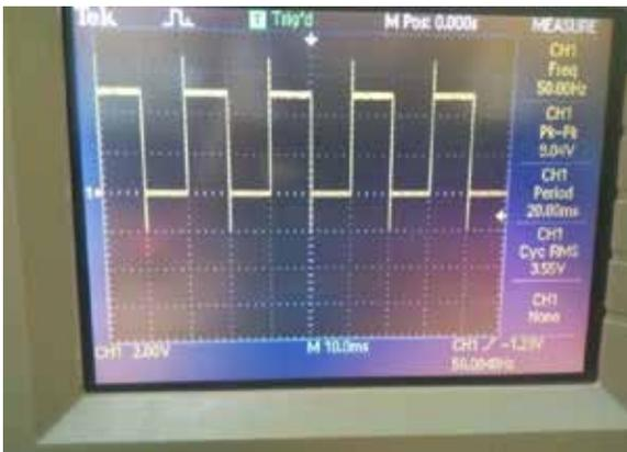
Figure 2 PWM pulse train for driver
