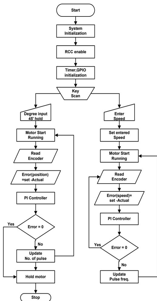
**Figure 6. Main program flow chart of implementation scheme**
