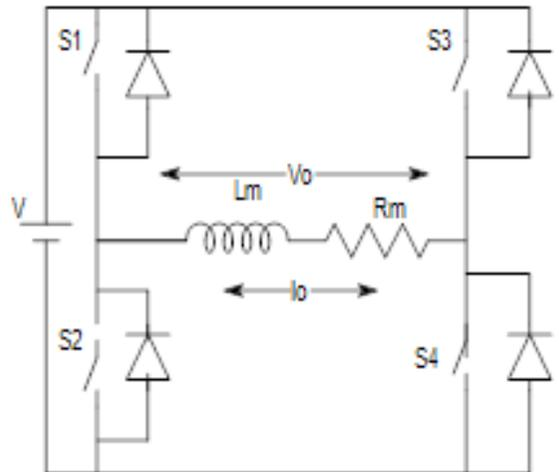
Figure 4 H-bridge driver for motor
