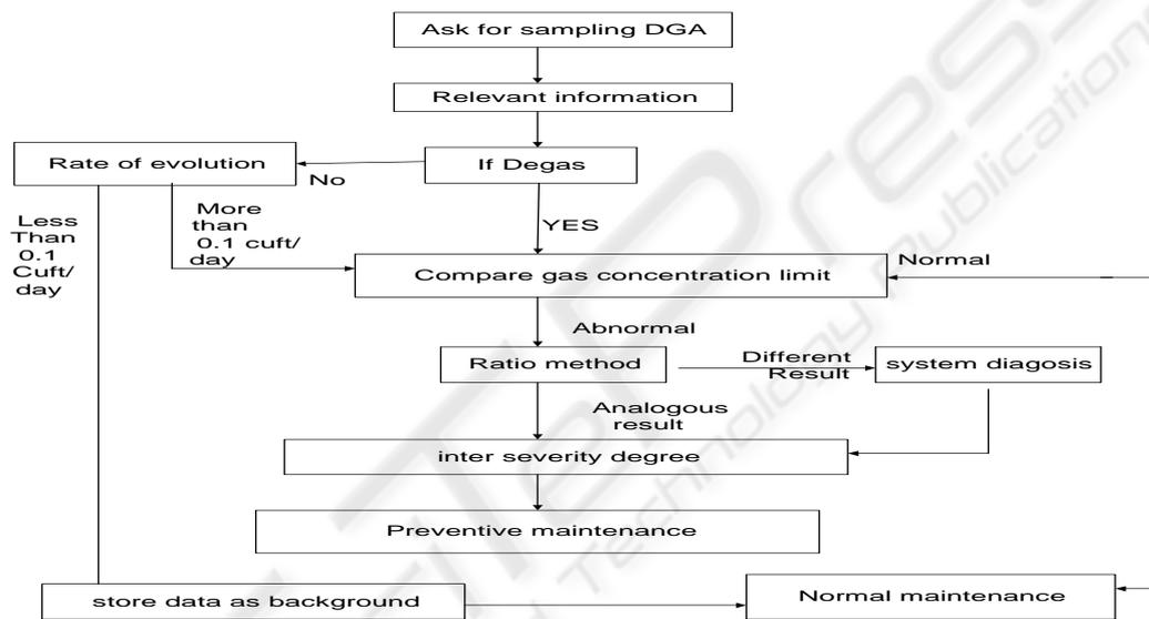
Figure 1: Procedure of proposed expert system
