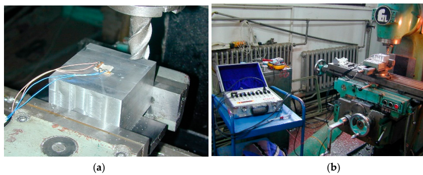
Figure 3. Quasi-nondestructive test for measuring distribution of residual stress. (a) Strain gauges and wire connecting; and (b) test equipment.
