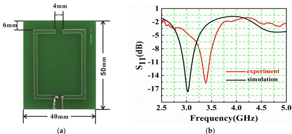
**Figure 2.** The split-ring based sensor. (a) Prototype board; (b) Experimental (red) and simulated (black, without Schottky diode) frequency response curves.
