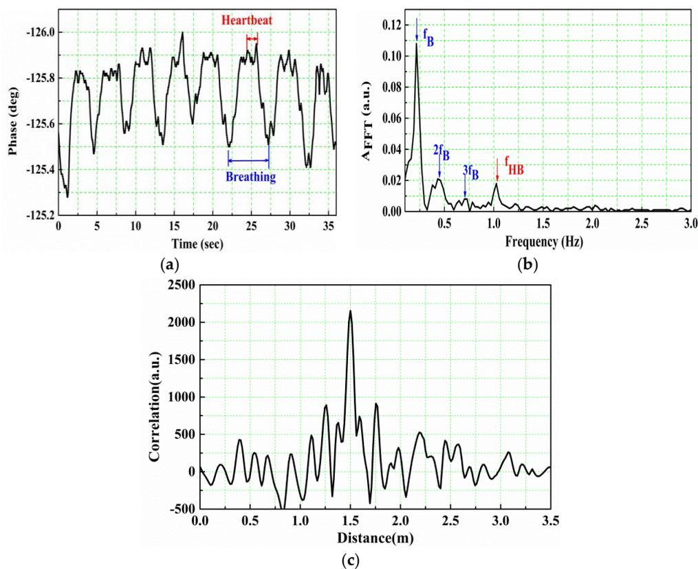
**Figure 4.** Experimental results of the target at the 1.5 m away from the antennas. (a) Raw phase data; (b) The FFT amplitude as a function of frequency obtained by performing FFT on the raw phase data; (c) Ranging result.
