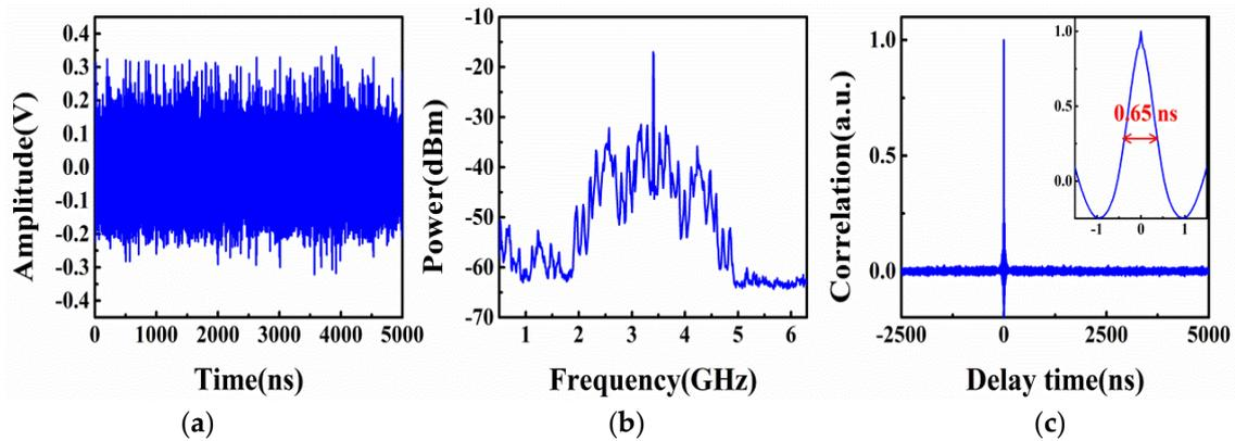
**Figure 1.** Properties of the transmitted signal. (a) Time series; (b) Power spectrum; (c) Autocorrelation trace.
