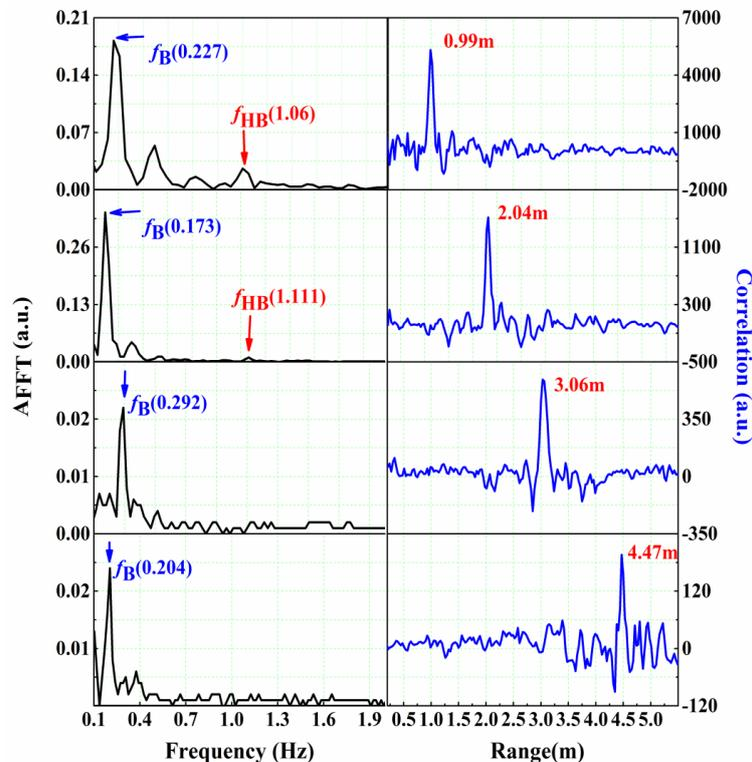
Figure 5. Experimental results in free space for human located at 1, 2, 3, 4.5 m.
