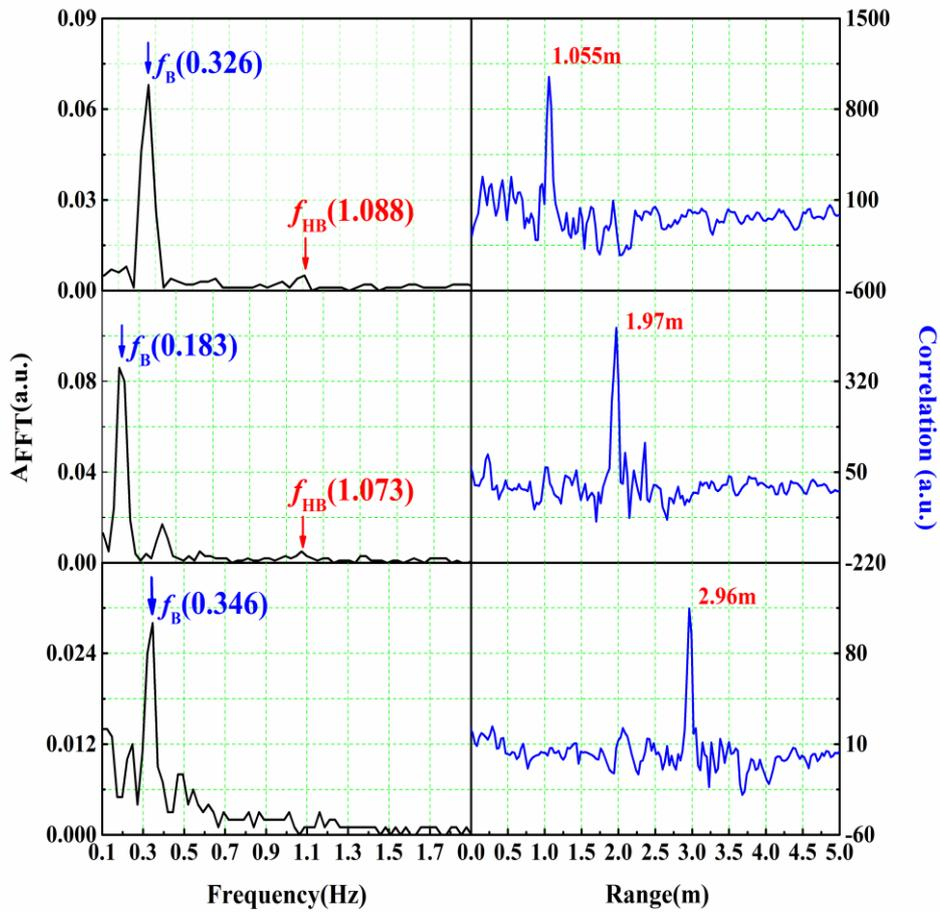
Figure 6. Experimental results with the cinder block wall for a human located at 1, 2, 3 m.
