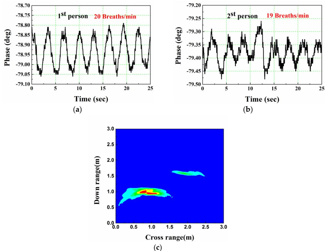
**Figure 10.** Human detection and imaging result for two human located at (0.8, 1.0) m and (2.0, 1.5) m, respectively. (a) Vital sign data of 1st human; (b) Vital sign data of 2nd human; (c) Two-dimensional imaging result.
