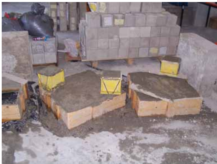
Figure 2. Specimens IS prepare by crushed limestone aggregate Mohs'hardness equal to 4.5
