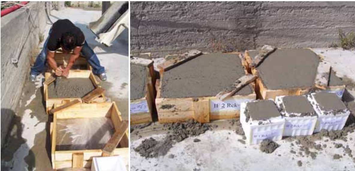
Figure 1. Specimens IF prepared by aggregates of fluvial origin - Mohs'hardness variable from 3 to 7 and equivalent Mohs'hardness equal to 3.15
