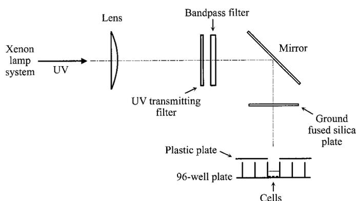
Fig. 2. Schematic experimental setup for UV exposure.
