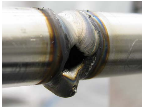
Figure 8. One of only two weld failures out of >260 welds. As ugly as it is, this weld represents a phenomenal overall success rate.
