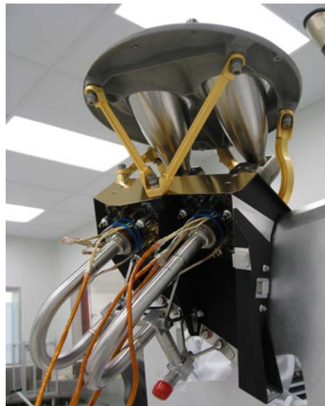
Figure 9. One of four RCS assemblies.
