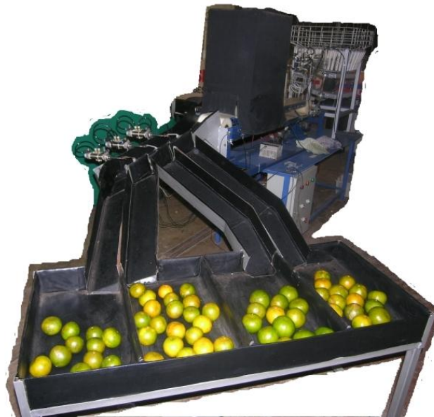
Figure 1. Automatic sorting and grading machine prototype for citrus
