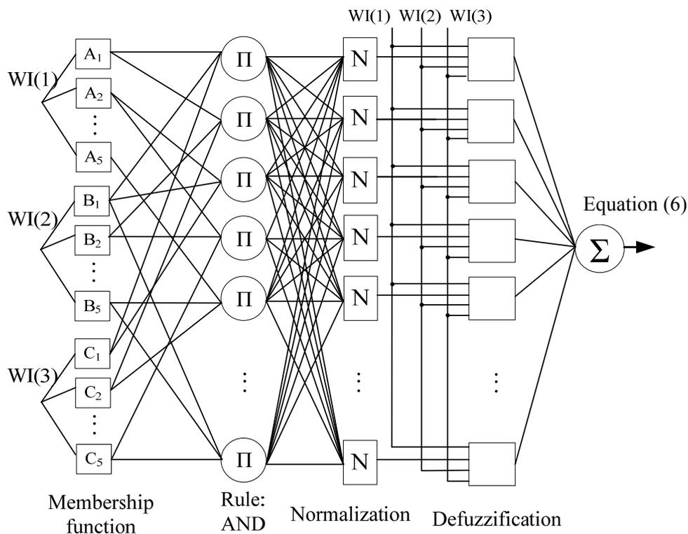
The structure of ANFIS can be explained as follows: the first layer in Figure 2 is the input layer; the second layer includes the membership functions, which are the same as the activation functions in the neural network, of the fuzzy rules. Each membership (activation) function can be expressed as follows:
