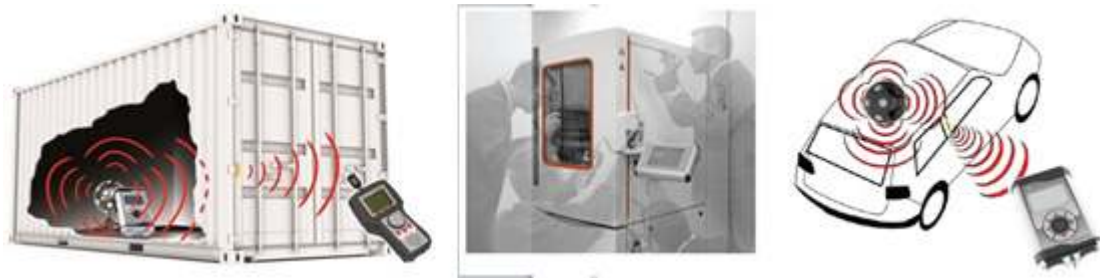
Fig. 4. Principles and several applications of the acoustic evaluation of tightness by means of an ultrasound active transmitter
