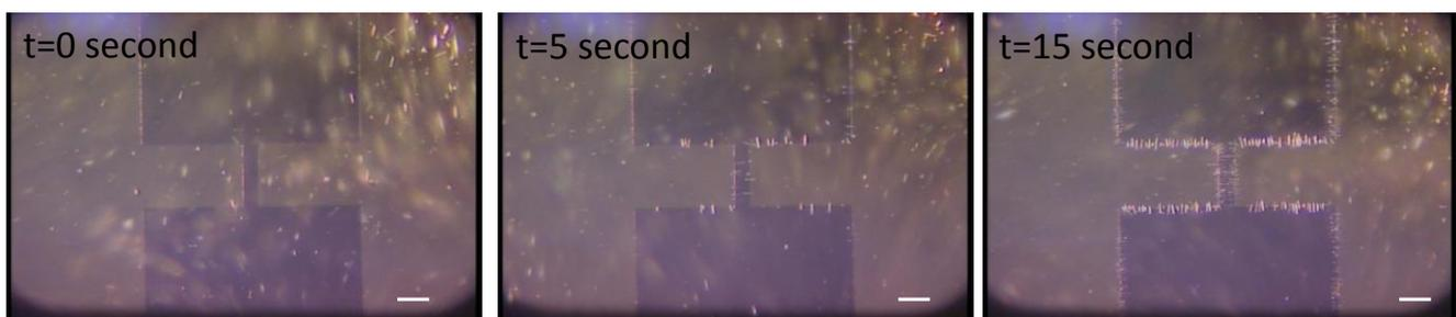
Considering the DEP force and torque, nanowires are attracted to a high electric field region with orientation. More polarizable and longer nanowires can be more easily attracted, which can be used for the selective deposition of nanowires. For demonstration of DEP, 10  $\mu\text{L}$  solution containing Si
