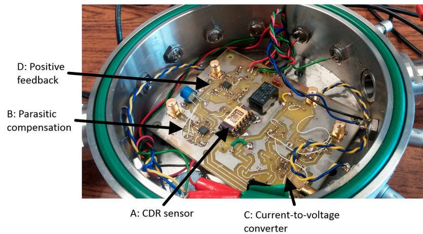
**Figure 3.** The CDR sensor and control circuitry.
