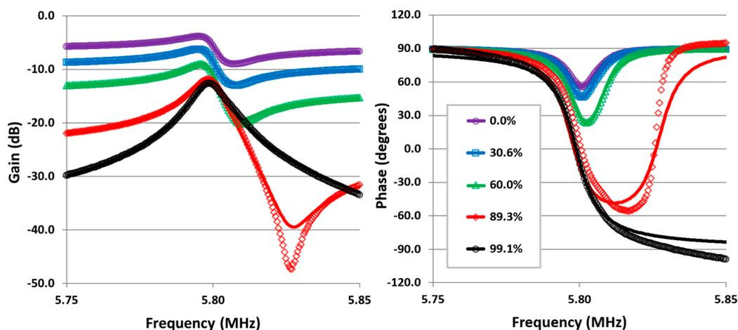
**Figure 5.** Amplitude and phase response traces for a CDR device. Legend refers to how much parasitic capacitance has been compensated for (100% corresponds to fully compensated). Points represent experimental data, solid lines represent a least squares fitted model—described by Equation (7)—to the experimental data.
