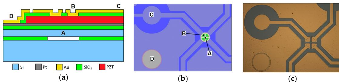
**Figure 1.** (a) Schematic cross section of the device (not to scale). ‘A’ indicates the resonator, ‘B’ is the top electrode contact, ‘C’ is the top electrode bond pad, ‘D’ is the ground plane electrode contact; (b) Screenshot of mask indicating lateral position of the features; (c) A microscope image of a fabricated device.
