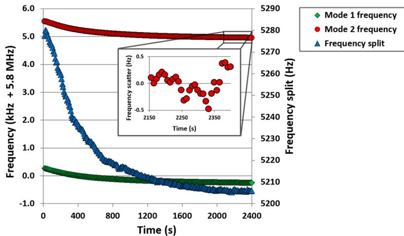
**Figure 8.** Frequency tracking tests of resonance frequency shifts induced by environmental temperature variations (green and red lines indicate resonance frequencies of modes 1 and 2 respectively, blue trace is frequency split between these modes). The scatter from a linear fit of mode 2 from 2150 s (inset) demonstrates resolution of frequency tracking is within 0.5 Hz.
