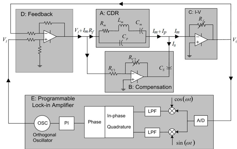
**Figure 2.** (Sub-circuit A): The equivalent circuit model of the CDR; (Sub-circuit B): Circuit used to compensate for the parasitic capacitance present; (Sub-circuit C): Current to voltage converter, nominal value of  $R_f$  is 100  $\Omega$ ; (Sub-circuit D): A current feedback scheme is used to increase the Q of the system; (Sub-circuit E): A digital lock-in amplifier arrangement (Zurich HF2) is used to track the resonant frequency.
