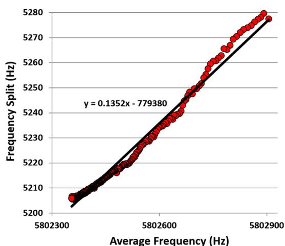
**Figure 9.** Frequency tracking tests of resonance frequency shifts induced by environmental temperature variations. Although frequency split should theoretically be temperature invariant, manufacturing tolerances result in a slight temperature sensitivity. As average frequency is highly indicative of temperature, this may be used to help compensate for temperature induced variations in frequency split.
