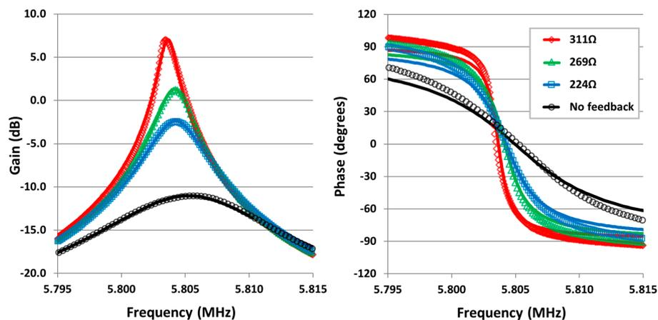
**Figure 6.** Frequency responses of piezoelectric based CDR with current feedback. Points represent experimental data, solid lines represent a least squares fitted model—described by Equation (9)—to the experimental data. Legend indicates values of feedback resistor  $R_f$ .
