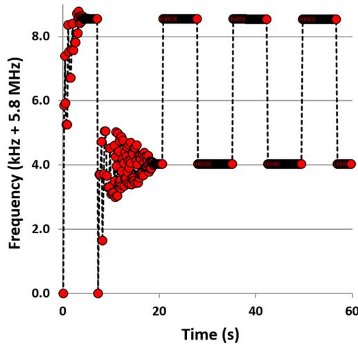
**Figure 7.** Frequency tracking is performed by phase-locking each mode. A mode is locked, the frequency is recorded and then the tracking system moves onto locking the other mode. This process continues to allow for assessing the frequency drift of each mode and allows for calculation of the frequency split. Once each mode is initially locked, relocating and locking takes approximately 7 s. The initial starting frequency is 5.8 MHz.
