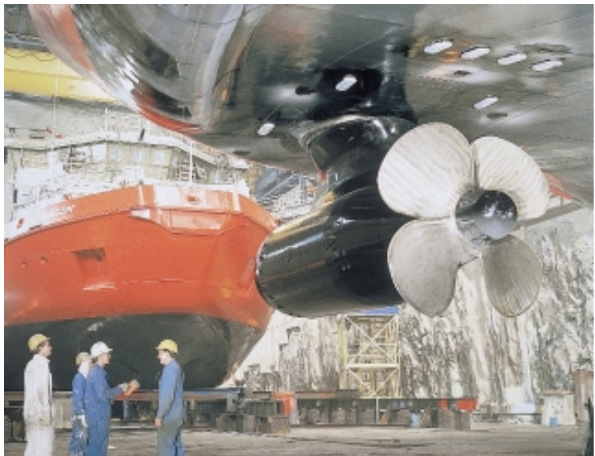
Arcticborg and Antarticborg ice-breaking supply ships, each powered by two 1,620-kW Azipod units, in the building dock. These vessels are driven stern-first when operating in severe ice conditions.
