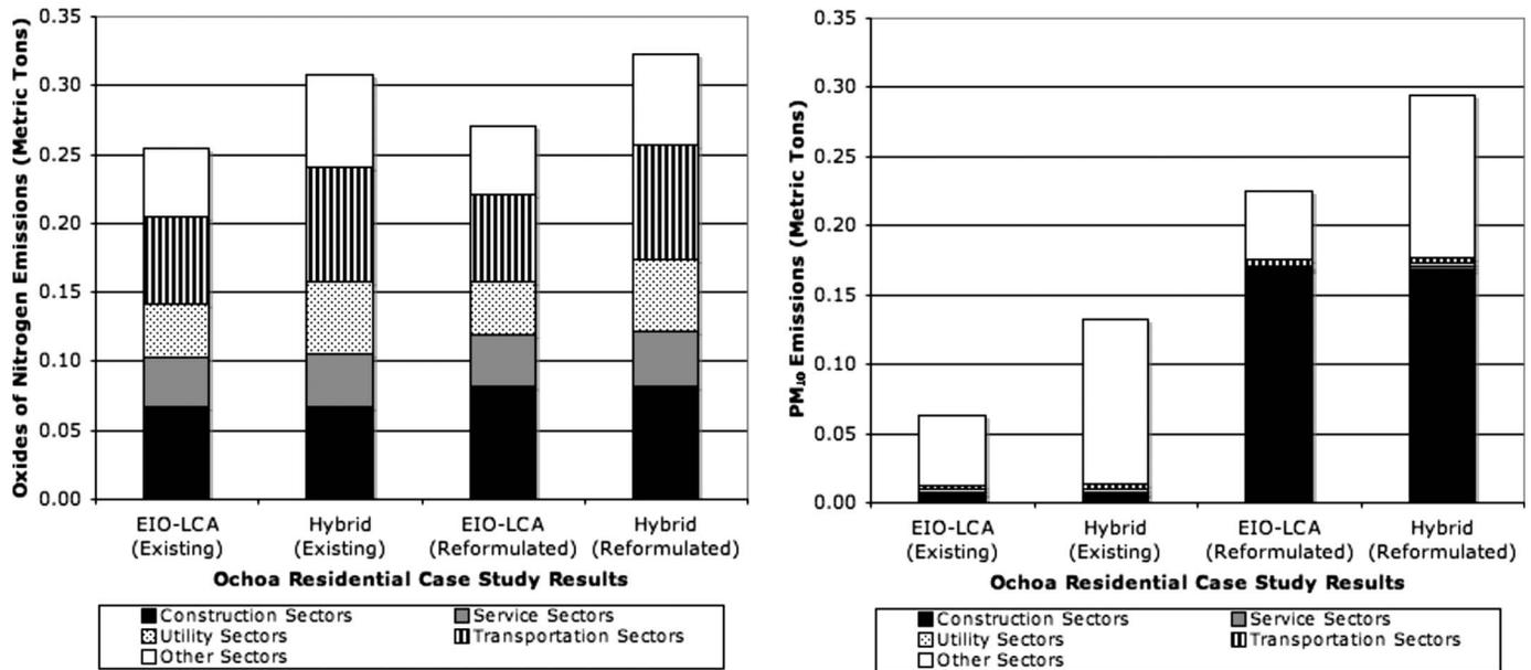
Fig. 2. Ochoa residential case study  $\text{NO}_x$  and  $\text{PM}_{10}$  I-O-based hybrid LCA model results
