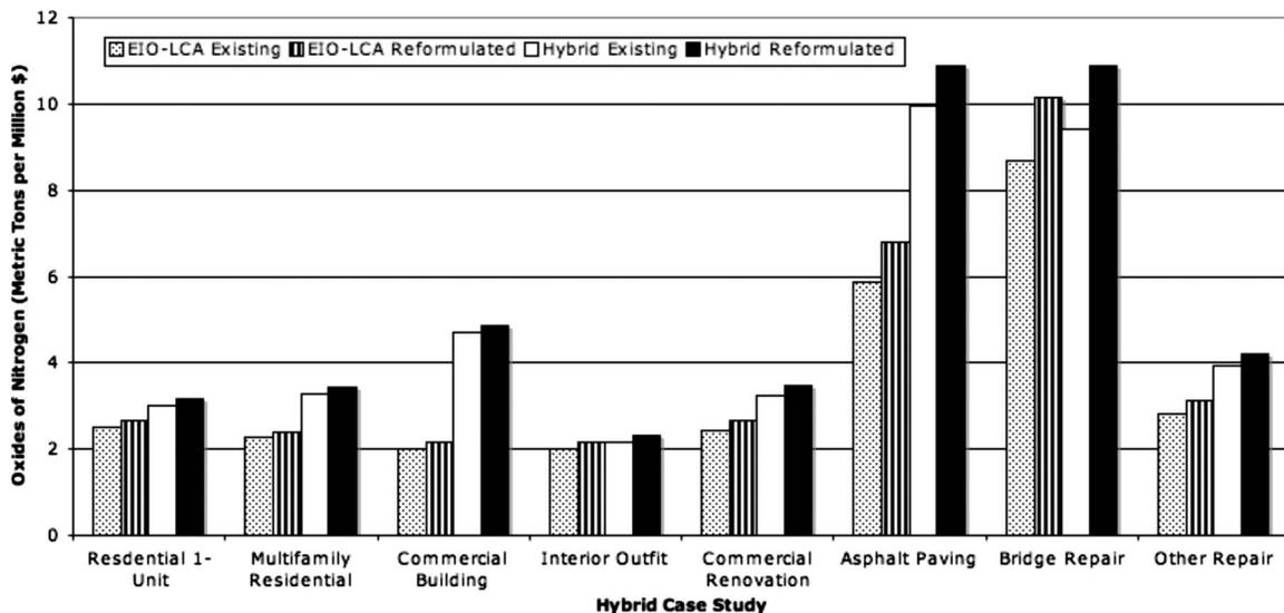
Fig. 5. Comparison of hybrid model NO<sub>x</sub> results for existing EIO-LCA and reformulated environmental effects
