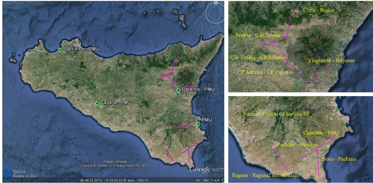
FIGURE 7: 150 kV lines object of reconductoring.
