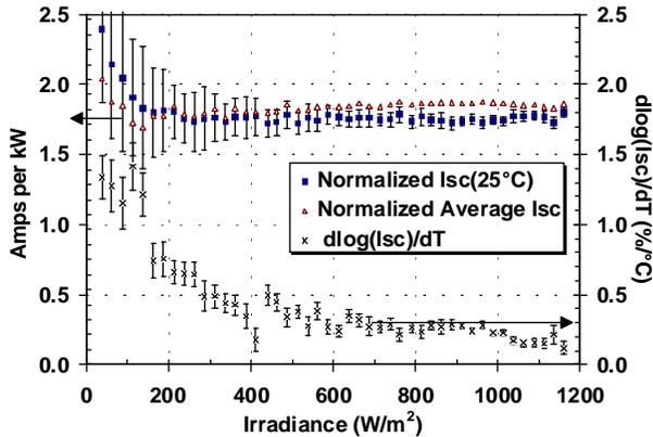
Figure 6. Irradiance-normalized Isc at 25°C (■) and average Isc (▲), and temperature coefficients(x) vs. irradiance, for Module 47-37. Error bars depict ± 1 standard deviation.
