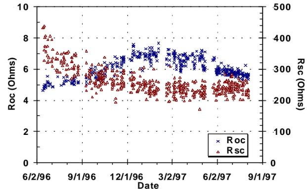
Figure 2. Module 47-37. Slope at open-circuit, Roc (x) and short-circuit, Rsc ( $\Delta$ ), plotted against time, for irradiances:  $1000 \text{ W/m}^2 \pm 5\%$ .
