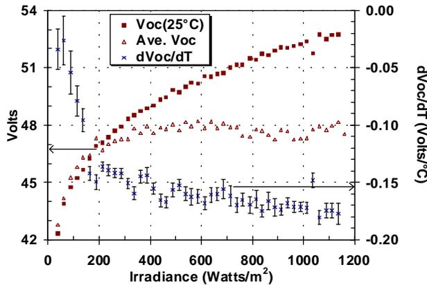
Figure 3. Module 47-37.  $V_{oc}$  at 25 °C (■), average  $V_{oc}$  (Δ), and temperature coefficients  $dV_{oc}/dT$  (x) plotted vs. irradiance.  $dV_{oc}/dT$  error bars depict  $\pm 1$  std. deviation ( $\sigma$ ).
