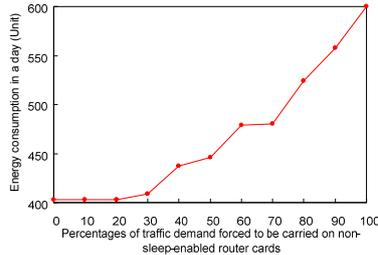
Fig. 5. Energy consumption in a day with different percentages of secured node pair capacity (n6s8).
