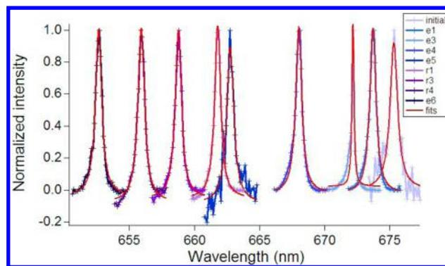
**Figure 4.** Controlled blue-tuning of a cavity mode via oxygen etching shown over eight etching steps. “e” refers to etching in an oxygen plasma etcher, while “r” refers to etch steps performed by annealing the samples in oxygen atmosphere in a rapid thermal processor. The etch times are of differing lengths, background has been subtracted, and modes are normalized by the peak intensity. An overall average tuning range of  $\sim 23$  nm was observed from several devices.
