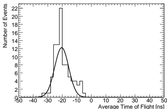
**FIGURE 1.** Time-of-Flight between D cells in back-to-back modules.
