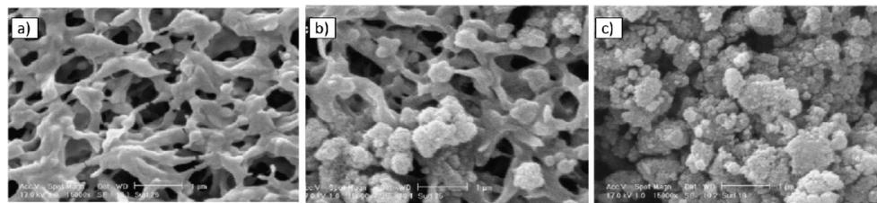
**Figure 4.** SEM images: (a) bare PVDF membrane; (b) PAA and self-assembling of TiO<sub>2</sub>; and (c) grafted by mixture of PAA and TiO<sub>2</sub>. Taken from [125].
