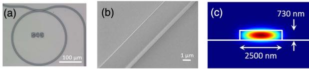
**Fig. 1.** Microscope images and mode simulation of the fabricated devices. (a) Top view optical microscope image of a 115  $\mu\text{m}$  radius ring resonator. (b) Scanning electron microscopy image of a fabricated waveguide with smooth surfaces. (c) Mode simulation of a 730 nm tall and 2500 nm wide waveguide showing the mode is highly confined in the geometry we have chosen.
