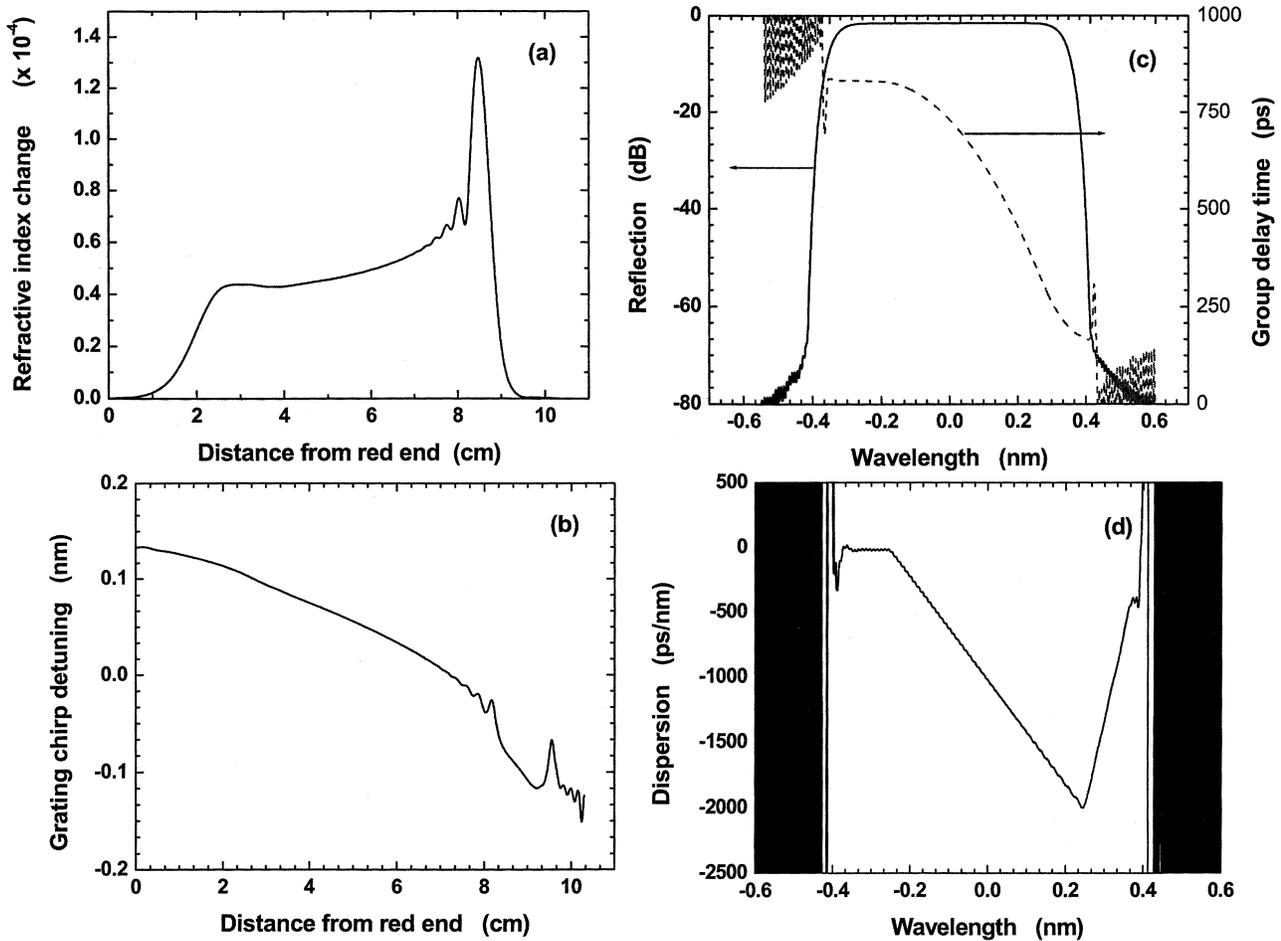
Fig. 8. Synthesized single-channel nonlinearly chirped FBG. (a) Apodization curve. (b) Grating chirp detuning. (c) Reflection and group-delay spectrum. (d) Dispersion spectrum.
