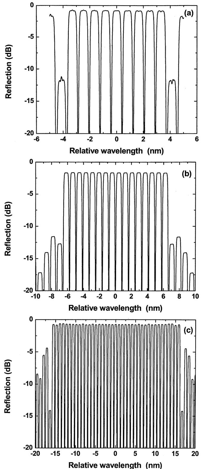
Fig. 5. Calculated reflection spectrum of the Dammann binary-phase-only sampled FBGs for (a) 9 channels, (b) 16 channels, and (c) 39 channels, with 0.8-nm channel spacing.
