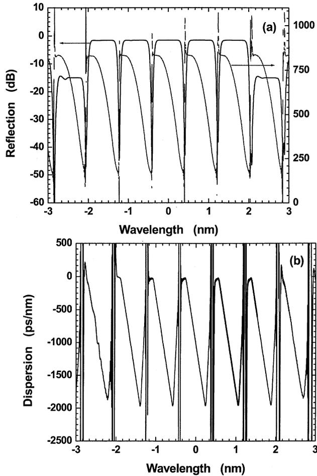
Fig. 9. Design of a five-channel nonlinearly chirped FBG using multilevel phase-only sampling function. (a) Reflection and group-delay spectrum. (b) Dispersion spectrum.
