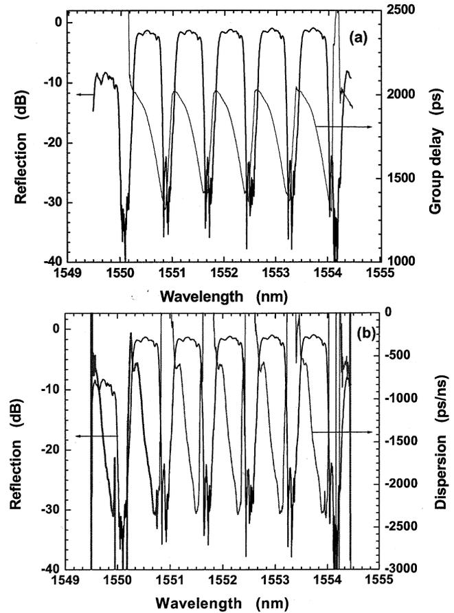
Fig. 10. Measured results of five-channel nonlinearly chirped FBG. (a) Reflection and group-delay spectrum. (b) Dispersion spectrum.
