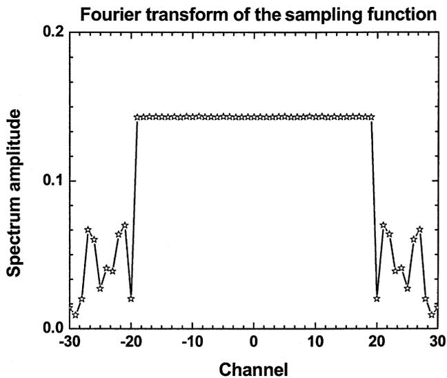
Fig. 4. Thirty-nine-channel binary-phase-only sampling function and its Fourier transform.
