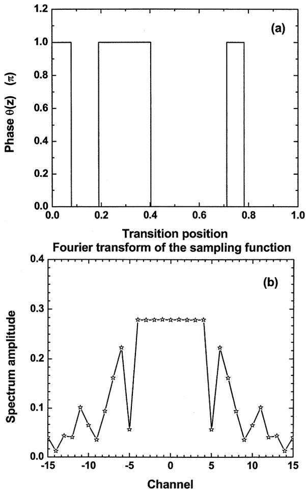
Fig. 2. Nine-channel binary-phase-only sampling function and its Fourier transform.
