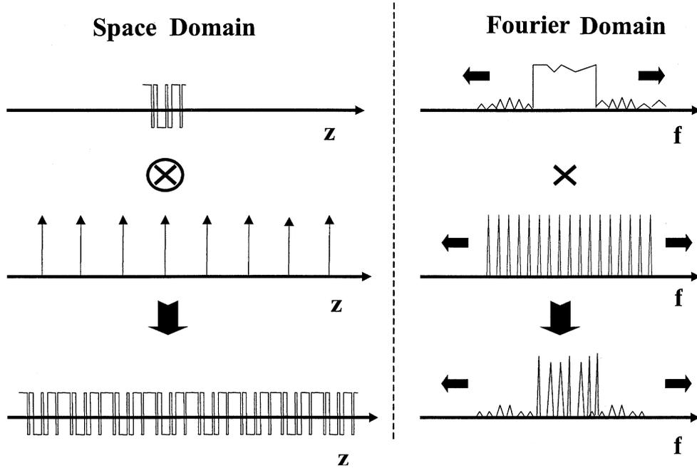
Fig. 1. Fourier analysis of a seven-channel binary-phase-only sampling function.
