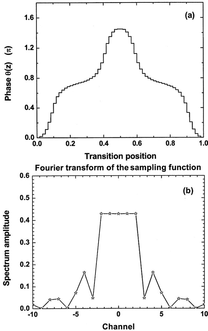
Fig. 6. Five-channel multilevel-phase-only sampling function and its Fourier transform.
