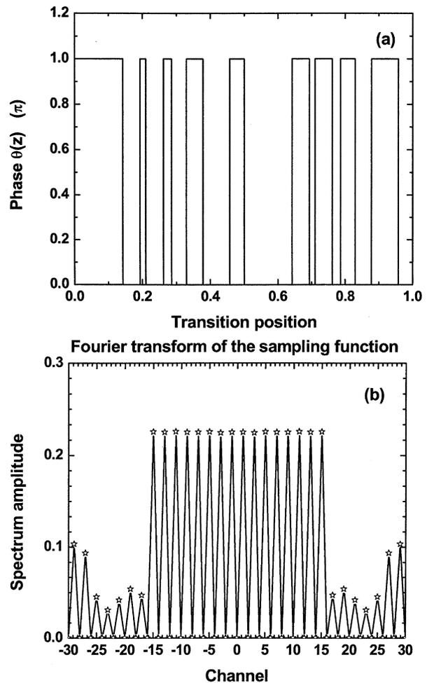
Fig. 3. Sixteen-channel binary-phase-only sampling function and its Fourier transform.
