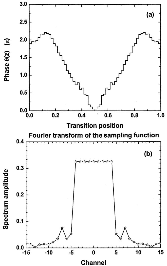
Fig. 7. Nine-channel multilevel-phase-only sampling function and its Fourier transform.
