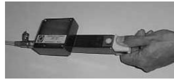
Fig. 4. The Pinch Force Dynamometer (Kayser Italia srl, Italy).
