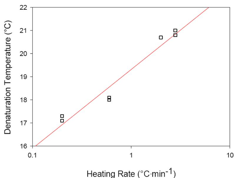
The collagen denaturation temperature increases logarithmically with heating rate [6,7,9]. The hoki collagen  $T_D$  also appeared to increase logarithmically with heating rate (Figure 3). This relationship
