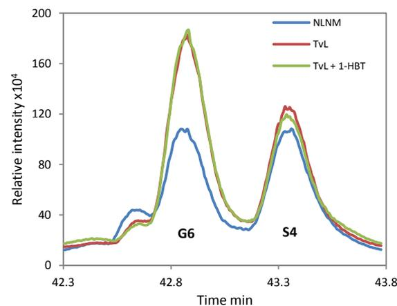
**Figure 2:** Partial chromatograms of the total ion current (TIC) for the TMAH thermochemolysis products methyl 3, 4, 5-trimethoxybenzoate (S6) (top), and methyl 3,4-dimethoxybenzoate (G6) and 3,4,5-trimethoxybenzaldehyde (S4) (bottom) for both laccase and laccase mediator treated wheat straw lignins and the untreated control.
