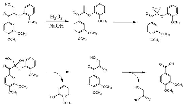
**Scheme 3.** The proposed pathway for the degradation of a phenacyl ether (involving cleavage of the C $\alpha$ -C $\beta$ ) by alkaline-peroxide treatment as investigated by Gierer *et al.*, [50]
