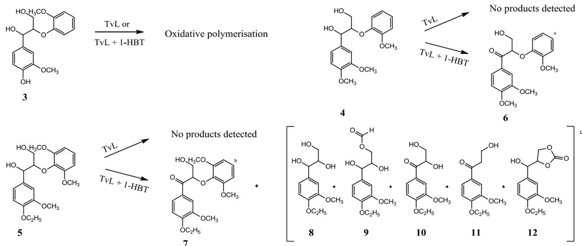
**Scheme 2:** Reactions of lignin model  $\beta$ -O-4 dimers **3**, **4**, and **5** <sup>a</sup> Product **6** characterised by MS and NMR following purification <sup>b</sup> Product **7** characterised by MS and by comparison with an authentic standard <sup>c</sup> Degradation products were identified by LC-MS and comparison with degradation products reported in the literature [40].
