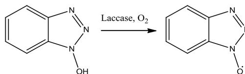
**Scheme 1.** The oxidation of 1-hydroxybenzotriazole (1-HBT) by laccase to produce the corresponding nitroxyl radical
