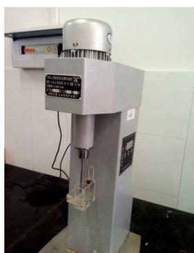
Figure 2. XFG flotation machine for a pure mineral flotation test.
