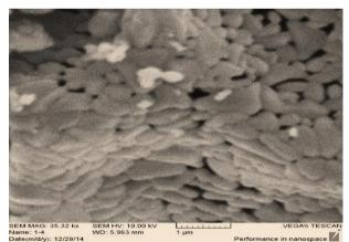
**Figure 1**: SEM images of α–Fe2O3 nanoparticles derived from oleic acid; after calcinations at 700°C through sol – gel method.
