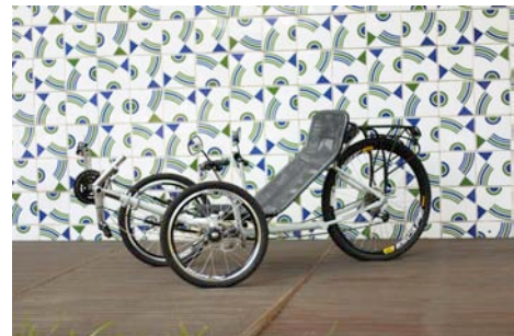
Figure 1. The tadpole Trike used in this work.
