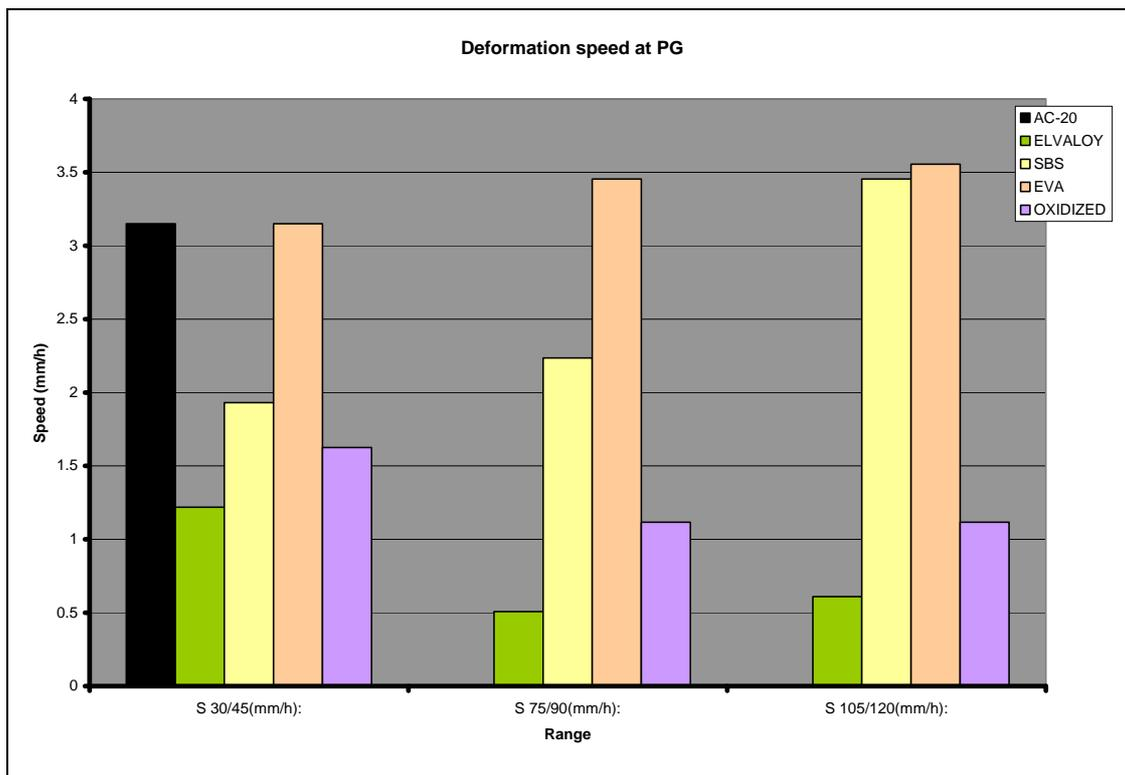
**FIGURE 3** Speed of deformation at high PG temperature for different mixtures (asphalts)
