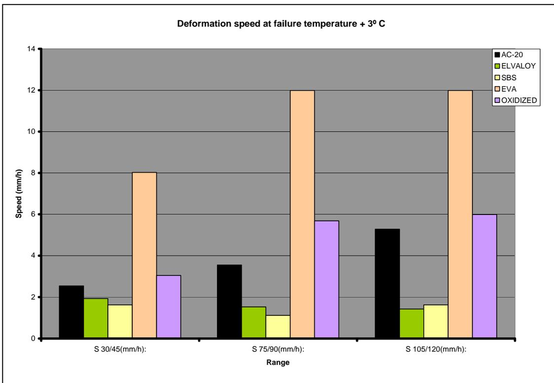
**FIGURE 4** Speed of deformation at failure temperature plus 3° C for different mixtures (asphalts)
