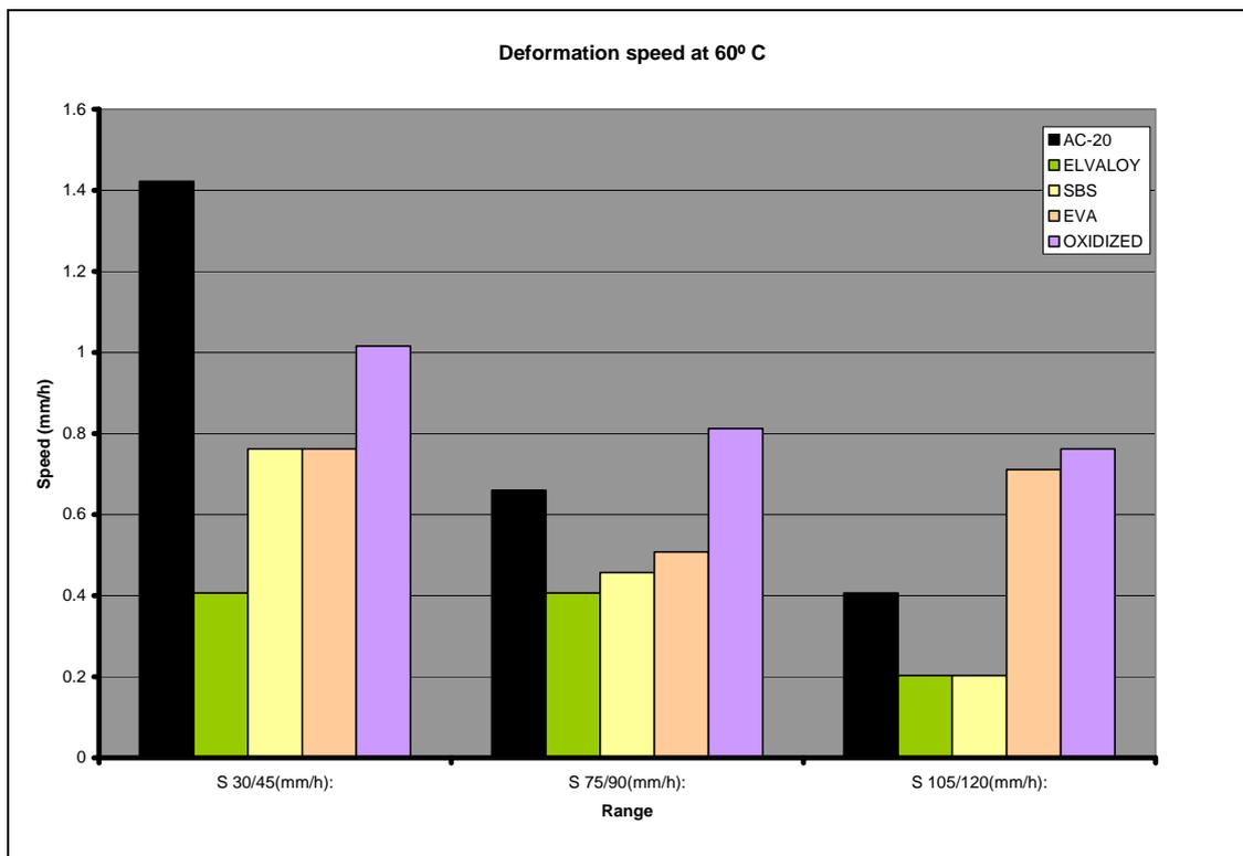
**FIGURE 2** Speed of deformation at 60° C for different mixtures (asphalts)
