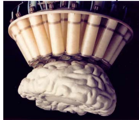
Fig. 13. BTi model 700C Neuromagnetometer® detection coils. Courtesy of Biomagnetic Technologies, Inc. San Diego, CA, USA.
