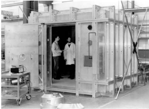
Fig. 15. Commercial magnetically shielded room showing first layer of mu-metal shielding and rigid aluminum frame. Courtesy of Vacuumschmelze GmbH, Hanau, Germany.
