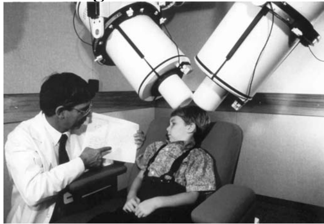
Fig. 1. A dual seven channel SQUID magnetometer used for magnetoencephalography. Courtesy of Biomagnetic Technologies, Inc. San Diego, CA, USA.
