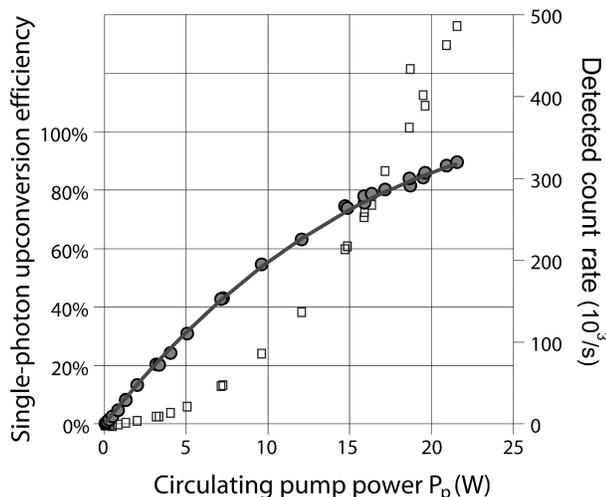
Fig. 3. Single-photon cw upconversion efficiency as a function of  $P_p$  (filled circles). Solid curve, functional fit of Eq. (3) with  $P_{\max} = 35$  W. Right axis, upconverted signal counts (filled circles) and background counts (open squares) as a function of  $P_p$ .
