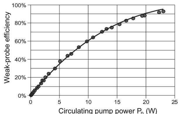
Fig. 2. Weak-probe cw upconversion efficiency as a function of  $P_p$ . Filled circles, experimental data; solid curve, functional fit of Eq. (3) with  $P_{\text{max}} = 31\ \text{W}$ .
