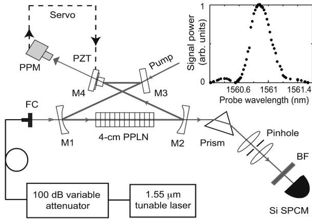
Fig. 1. Experimental setup for single-photon detection at  $1.55\ \mu\text{m}$  by means of upconversion. FC, fiber-optic collimator; BF, 10-nm interference filter at  $633\ \text{nm}$  and  $1064\text{-nm}$  HR mirror; PPM, pump power monitor; PZT, piezoelectric transducer. Inset, wavelength phase-matching curve at a PPLN temperature of  $229\ ^\circ\text{C}$  ( $\sim 0.3\text{-nm}$  bandwidth).
