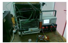
Fig. 5. Self oscillated induction heater and absorption cooler.
