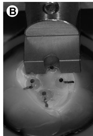
Figure 1. Loading devices. A: Knife-edge. B: Notched rod.
