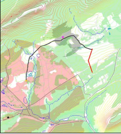
Figure 8. Path calculated with all weights set to 1. This path is a compromise solution that tries to achieve low mobility risk, short time, low exposure and high coverage.
