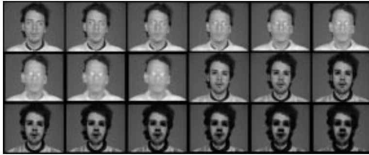
Fig. 1. Dilated and eroded images with a scaled hemisphere for scales 1–9.
