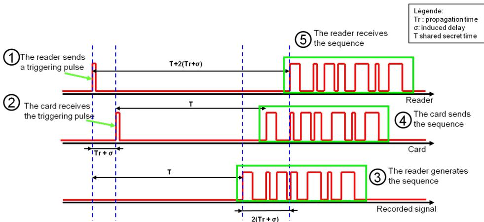
**Figure 6.** Time measurement stage in the proposed protocol
