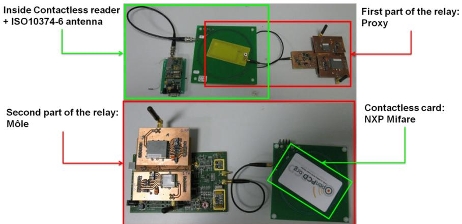
**Figure 4.** Relay with demodulation of the signal
