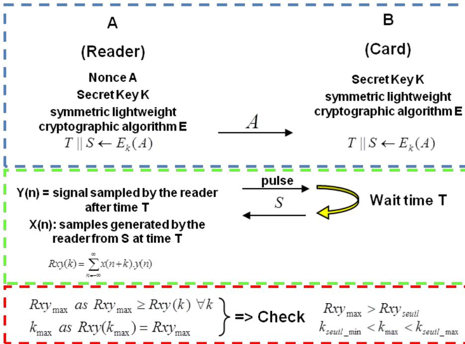
**Figure 7.** The proposed protocol consists of three stages. The first stage calculates two pseudorandom numbers, using a symmetric cryptographic algorithm and a secret key  $k$  and an exchanged nonce. The second stage is time critical as the card has to answer one of the generated pseudorandom sequences, a time  $T$  after a synchronization pulse. The third is the verification of the relay presence
