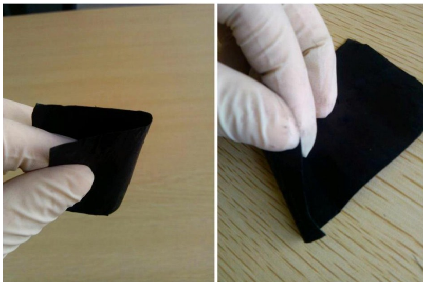
Figure S2. Photographs of carbon nanotube film. (Provided by Yijie Technologies Co., Ltd. (Shanghai, China))
