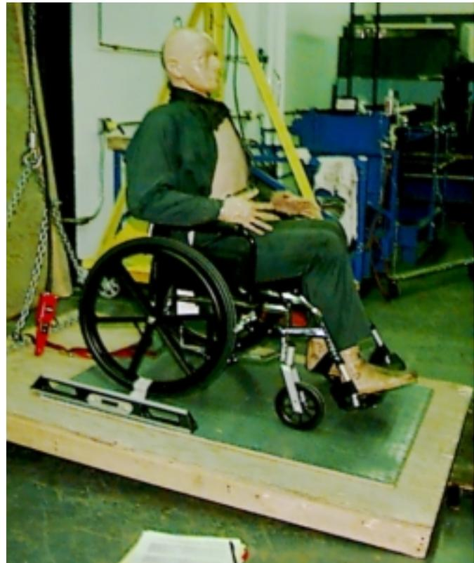
Figure 54 - Sliding test procedure using tilt platform
