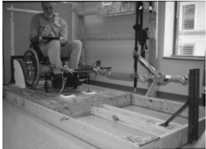
Figure 51 – Pull testing set up of the low “g” prototype securement device
