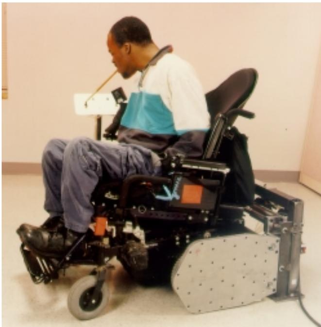
Figure 50 – Low “g” Docking System Securing Power Wheelchair
