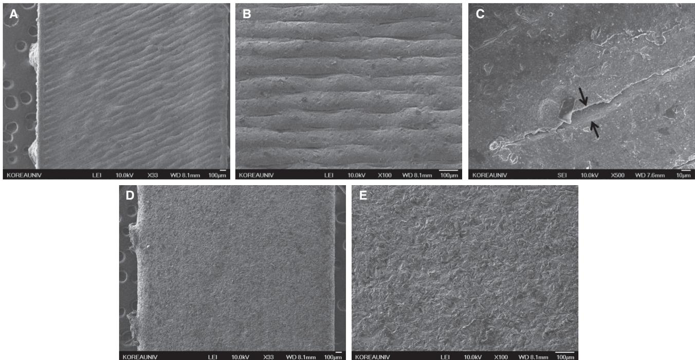
**Fig. 1.** SEM images of SLS specimens magnified at  $\times 33$  (A),  $\times 100$  (B), and  $\times 500$  (C) and of CAST specimens at  $\times 33$  (D) and  $\times 100$  (E). The black arrow was the spacing between the layers (about 10-20  $\mu\text{m}$ ).
