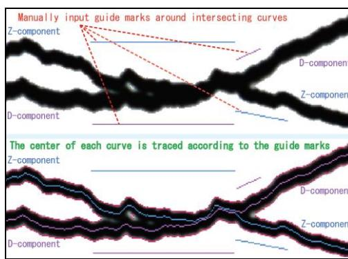
**Figure 3.** Identifying two curves at an intersection
