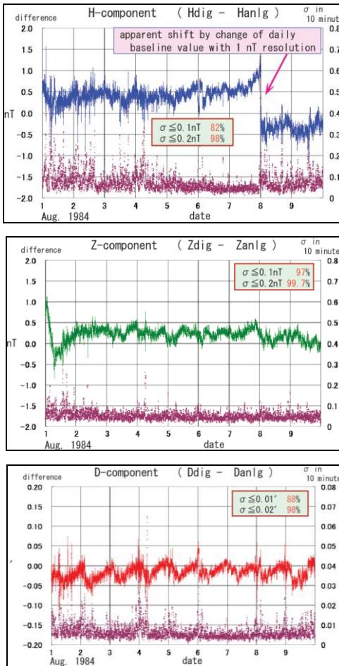
**Figure 5.** Differences in each component between the digital one-minute values and converted analog one-minute values (upper trace in each panel) and standard deviations computed using one-minute difference values determined over each 10-minute interval (lower trace in each panel)
