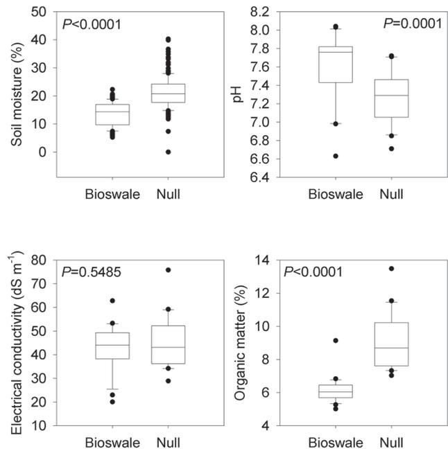
Fig. 1. Soil moisture, pH, electrical conductivity, and organic matter (0–25 cm) in bioswales of The Morton Arboretum parking lot and adjacent nonbioswale (null) locations. \*  $P < 0.05$ .
