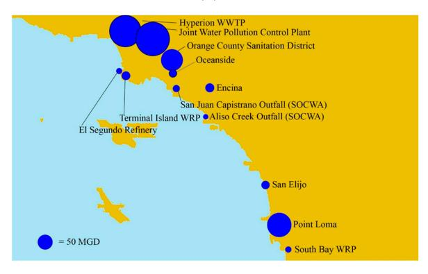
**Figure 7.** Location and average dry weather effluent flow rates of WWTFs in the South Coast region that discharge at least 3.8 MLD (1 MGD).
