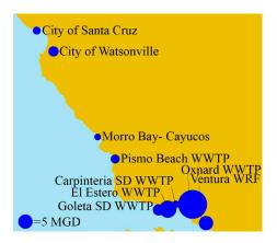
**Figure 6.** Location and average dry weather effluent flow rate rates of WWTFs in the Central Coast region that discharge at least 3.8 MLD (1 MGD). WRF, Water Reclamation Facility.
